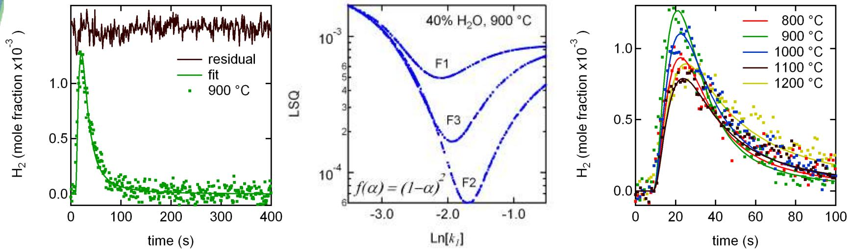
$$\frac{d\alpha_1}{dt} = k_1 [Y_{\text{CO}_2}^0 (t - t_{\text{shift}})] \cdot f(\alpha_1)$$
