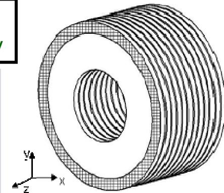
Counter-Rotating-Ring Receiver/Reactor/Recuperator (CR5)
