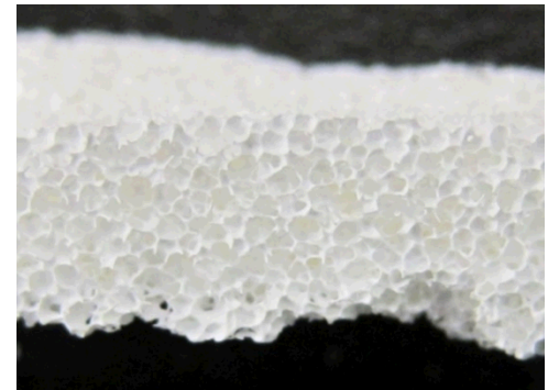
Sintered samples of replicated ceramic foams
