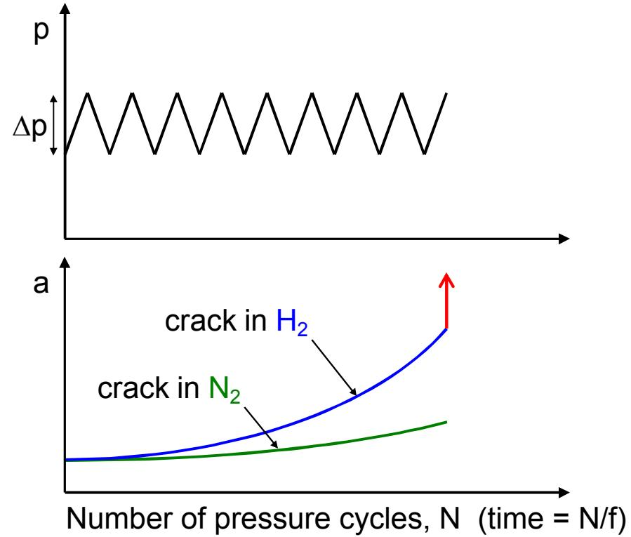
Fatigue crack growth followed by rapid failure
