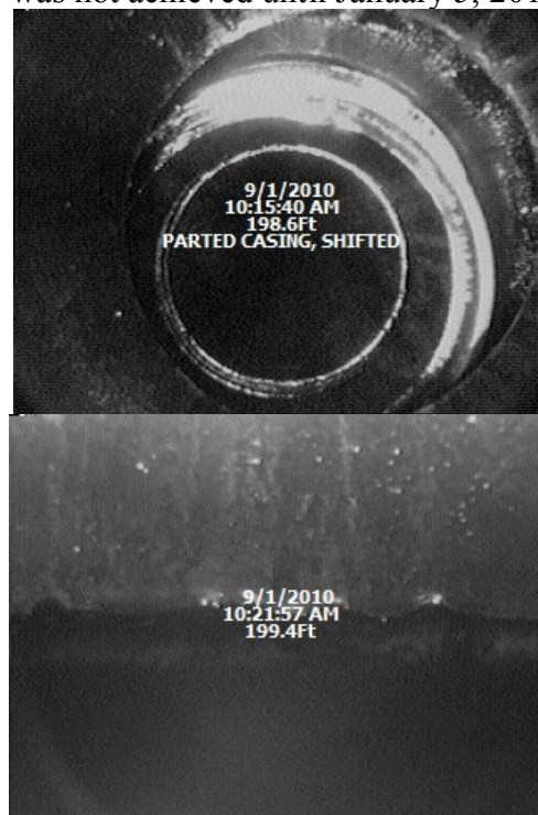
Figure 3. Camera shots showing parted casing (upper- looking down well, lower- sidewall image) just above collar at 60.8 m (199.5 feet) (courtesy DM Petroleum Operations Co.).
