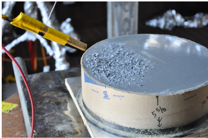
Figure 3: Igniter and Propellant Sample on Test Bed
