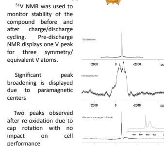
We investigated a series of polyoxometalates (POMs), as a new dissolved charge storage material. POMs are nanometer-size analogues of metal-oxide lattice with an array of attractive attributes including solubility in non-aqueous solvents, which is of interest for new battery materials.
