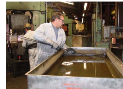
Transfer to quench bath (~3 to 5 sec)
