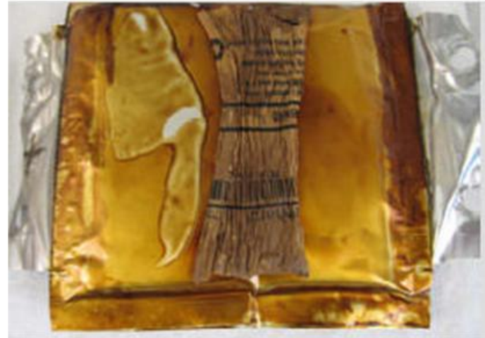
Photo 3. High temperature testing results; Left – Traditional Li-ion battery; Right – nLTO-based battery (note the nLTO battery did not explode)
