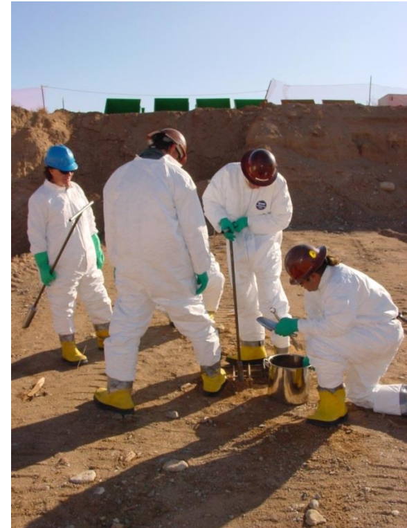
Verification sampling of excavation floor
