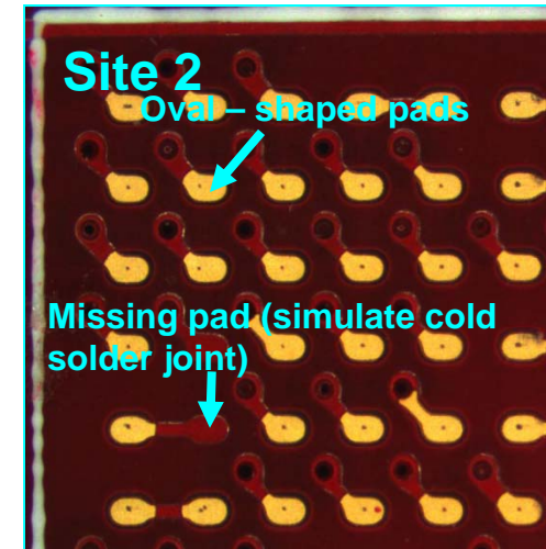
Magnified view of sites 1 and 2 showing the intentional defects
