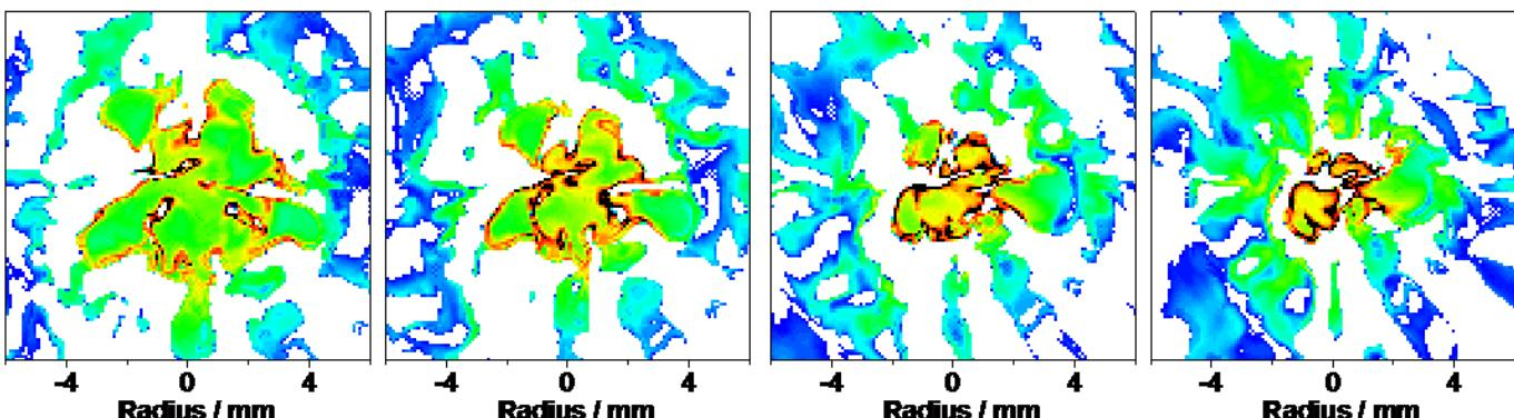
Rise of K-shell x-ray pulse is more like snow plough radiation as pinch collapses.
