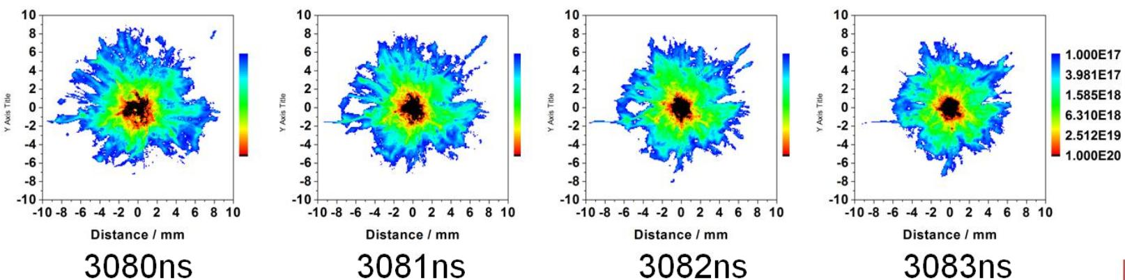
Unstable disassembly of pinch, when viewed in emission and integrated along axis appears like a stable pinch in pressure balance, but the finite pinch size is not maintained by pressure balance, but by a failure to geometrically converge
