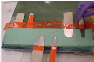
Pull tabs in bond joint
