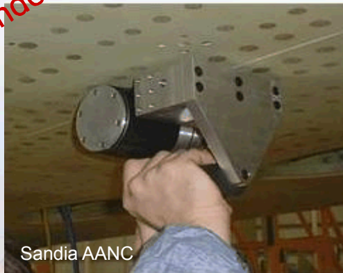
Phased Array UT Inspection of an Aircraft Vertical Stabilizer Specimen
