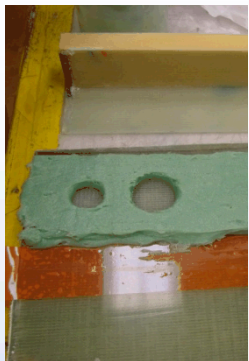
Voids in bond joint
