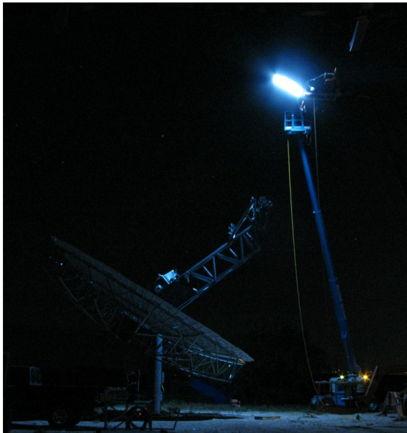
Figure 2. AIMFAST elevation-dependent measurement of SES dish. The LCD TV screen and camera are located on a forklift near the 2f point.
