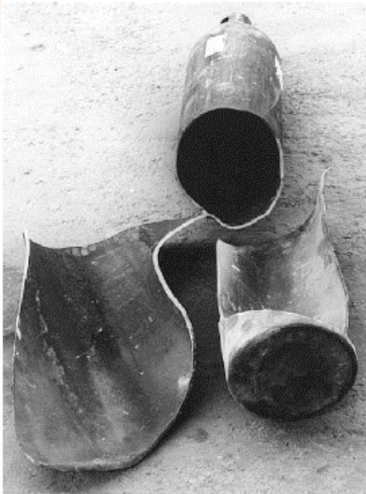
Hydrogen-induced failure of transport cylinder
