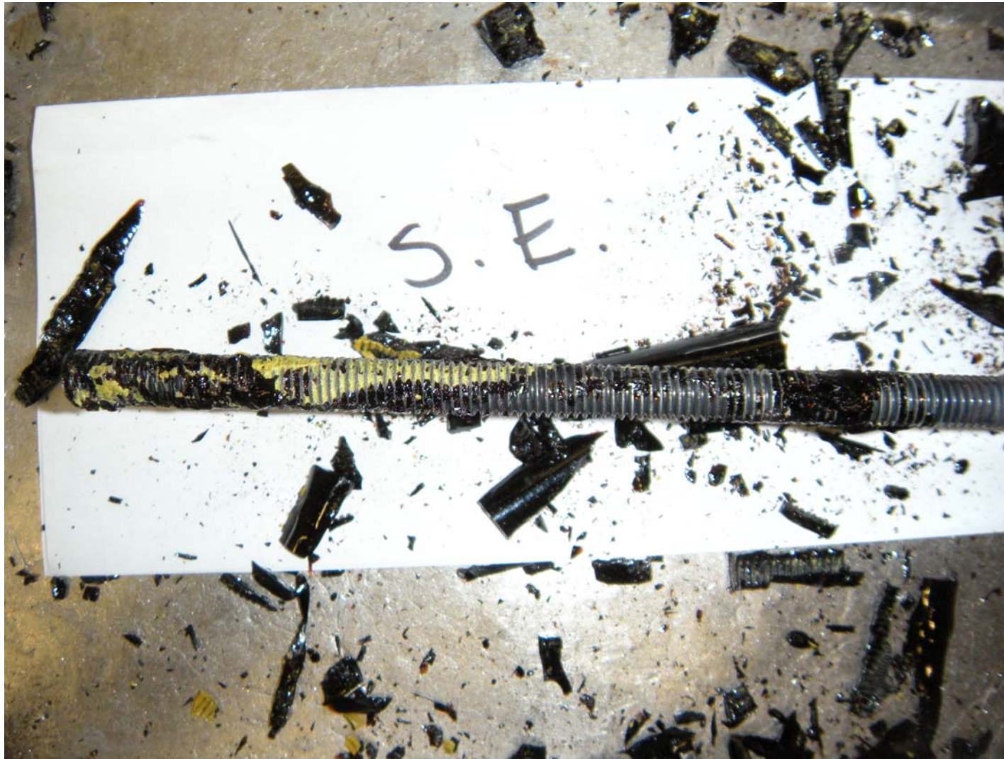
Figure 5.6(b). Secondary phase observed on dip sample, D-10B-67C, taken after Test 2D.
