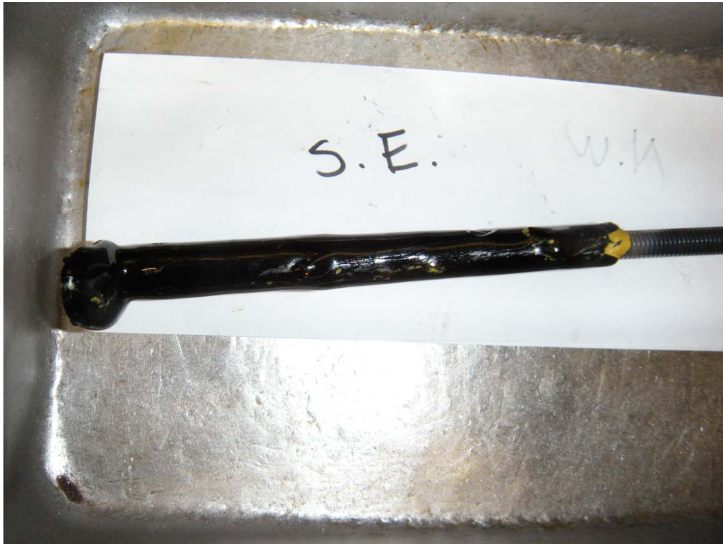
Figure 5.6(a). Secondary phase observed on dip sample, D-10B-67C, taken after Test 2D.
