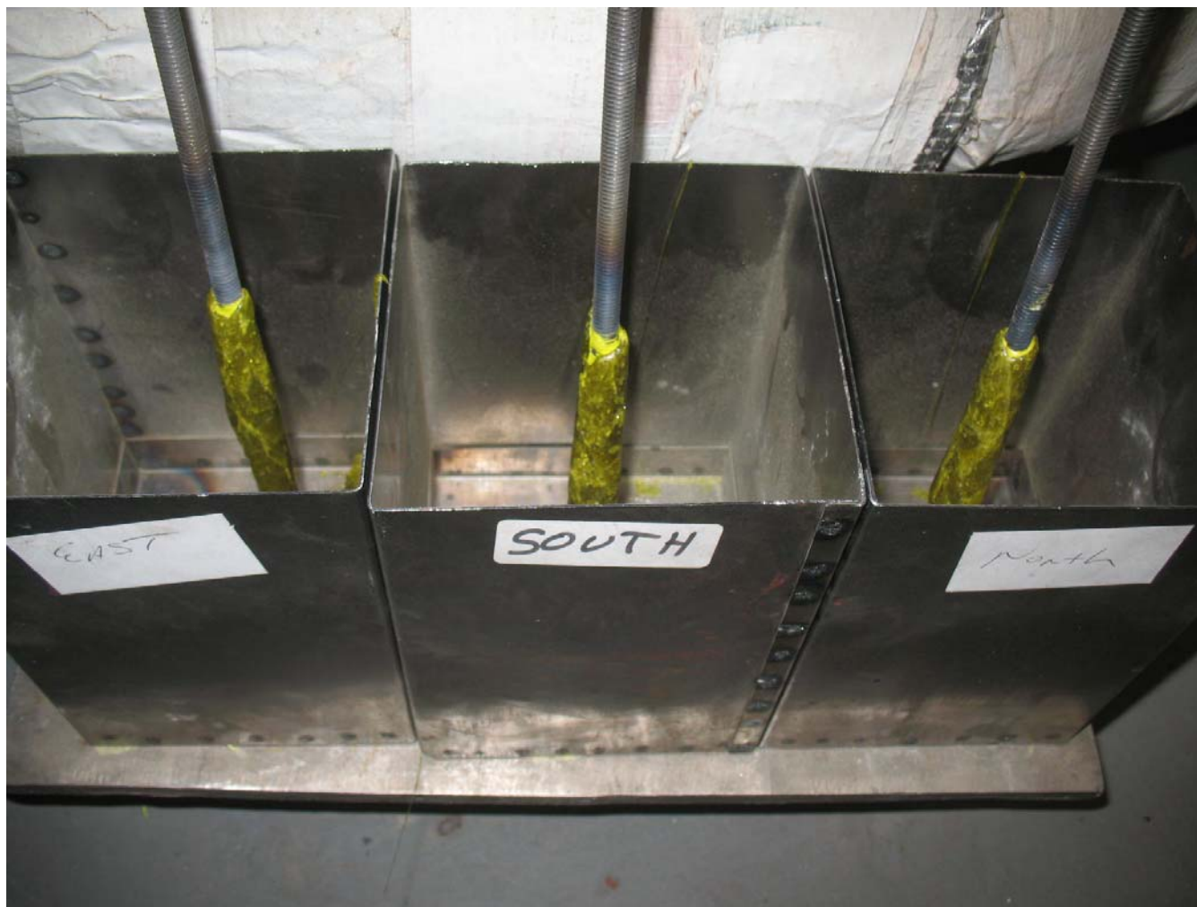
Figure 4.15. Secondary sulfur phases on dip samples S10-D-110A, B, and C from the end of Test 4D.
