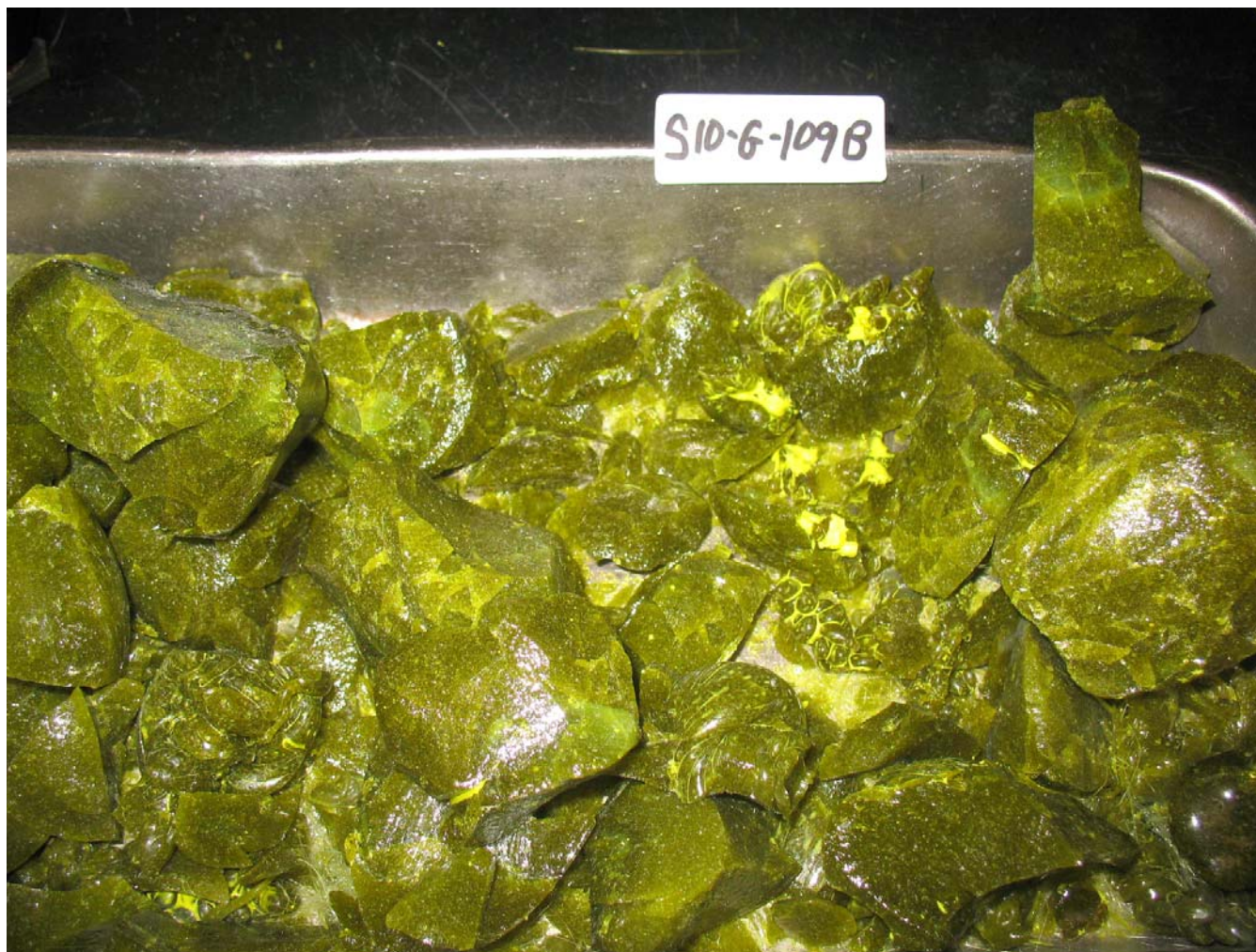
Figure 4.1. Secondary sulfur phases on discharge glass S10-G-109B from the end of Test 4D.
