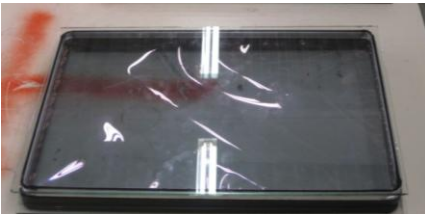
Figure 4: HM IGU with experimental polymer warm-edge spacer prior to sealing and tensioning
