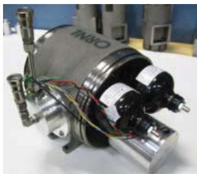
FIGURE 16 Additive manufactured hydraulic power unit with motor, pump and accumulators.
