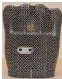
FIGURE 12 Meshed palm weighing 178 grams.
