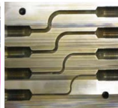
FIGURE 3 Cross-section of the test manifold.
