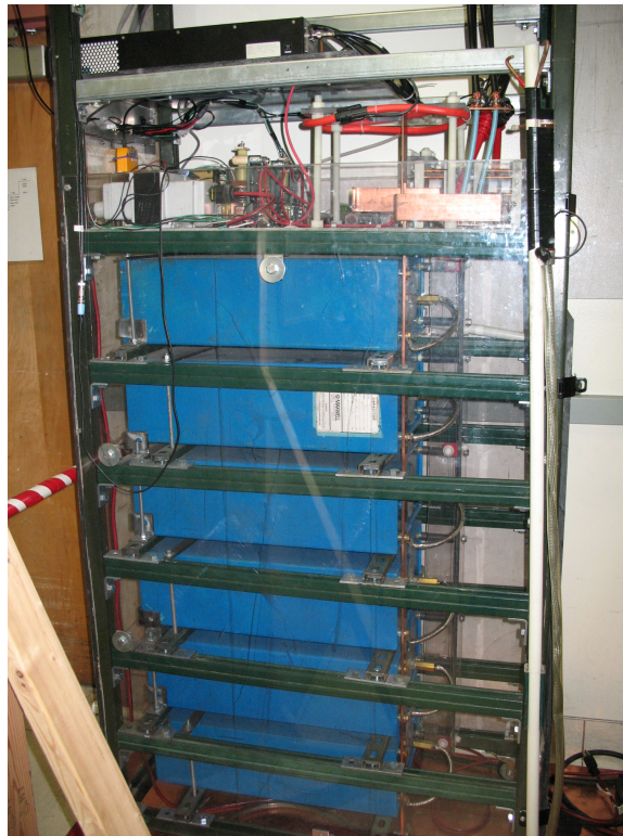
Figure 2: Capacitor bank for driving solenoid magnet
