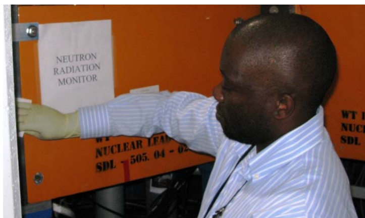
Figure 2-2. Example of a Point ES at a Beam Stop at a Suspected Enrichment Laser Facility in a Training Exercise at Brookhaven in 2010
