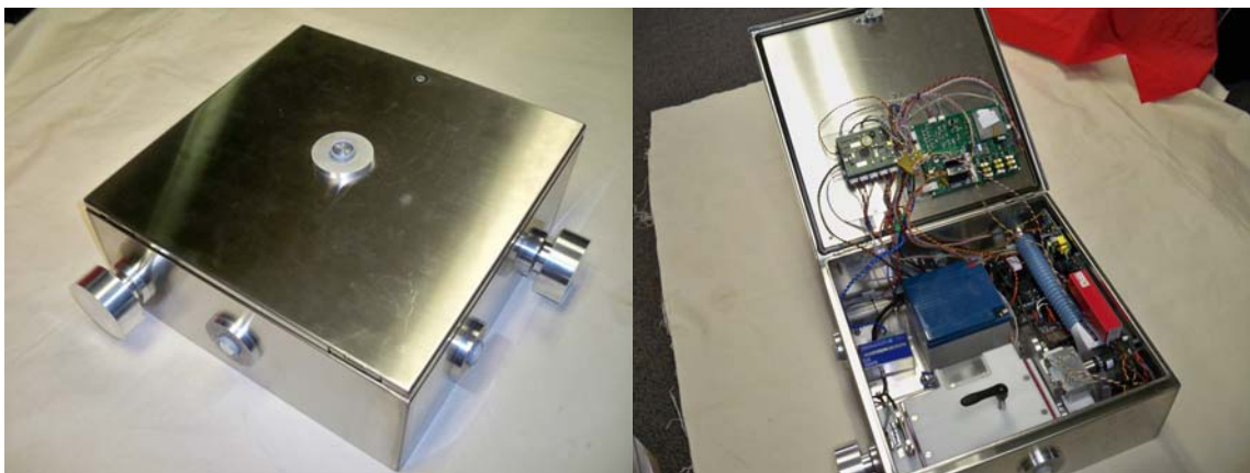
Figure 3-5. TRI-ACE Prototype Outer Enclosure (left), Components Inside the TRI-ACE Prototype (right)
