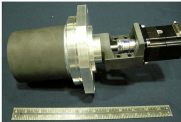
Removable impactor drum with motorized rotation assembly
