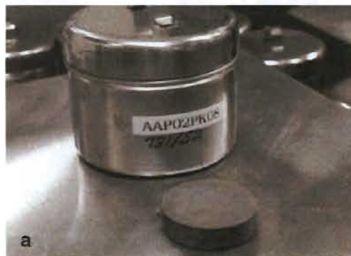
plutonium aging Pu-238 accelerated-aged ingot
