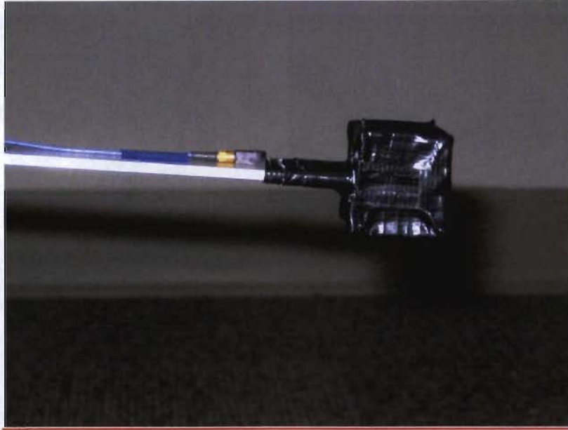
Figure 4. Mass attached at tip to help drive geometrically nonlinear deformation.
