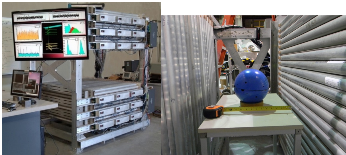
Figure 28) Left: photograph of the muon scanner in vertical viewing mode. Right: photograph of the scanner in horizontal viewing mode with the lead sphere in place.
