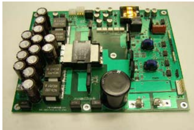
Figure 50: 24V Aux and Module – Heat Sinks not Installed
