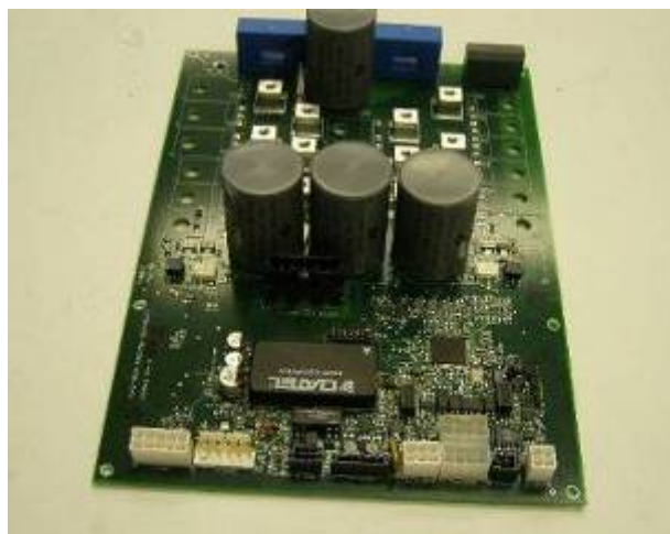
Figure 51: Application Controller/Boost Flyback Board
