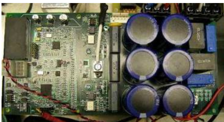
Figure 52: Inverter Controller Board
