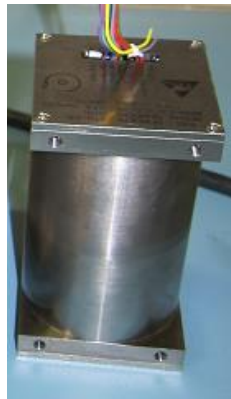
Figure 2.5.1.5 shows the physical characteristics of the ARS24 sensor. The sensor package is approximately 2"x2" at square ends and 4 inches long.
