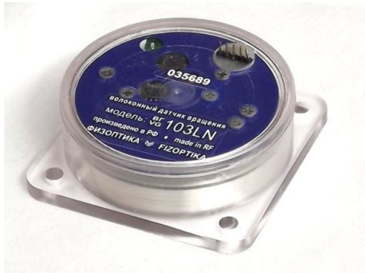
Figure 2.5.1.7 shows the Fiber Optic Gyro model VG 103LN rotation rate reference sensor. The physical dimensions of the sensor package is approximately 2.5"x2.5" at square ends and 0.8 inches thick.
