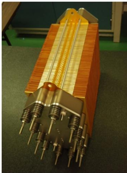
Figure 1. One of EnerFuel's early air-cooled HTPEM stacks with gold coated stainless steel bipolar plates.
