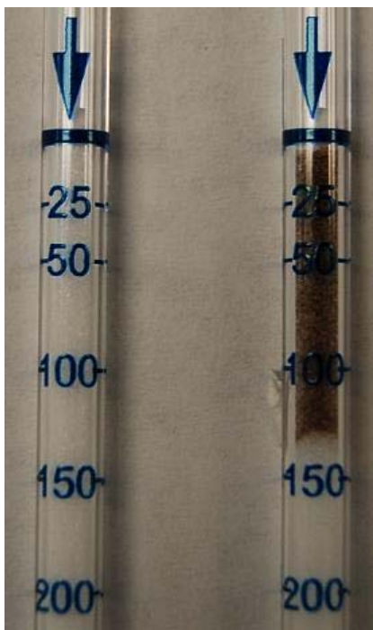
Figure 33. Analysis of H 2 S in pre-reformer effluent using Sensidyne™ gas detection tubes.
