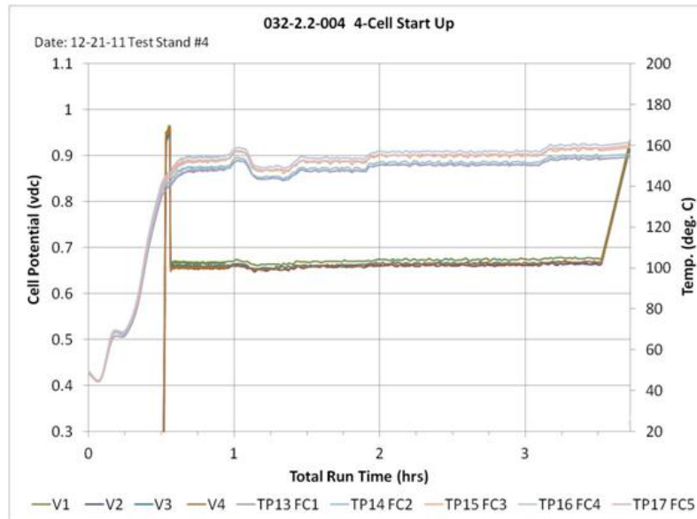
Figure 18. Baseline test data showing the voltage and temperature of each cell in EnerFuel's baseline 4-cell stack (with pre-HiFoil™ bipolar plates comprising an experimental expanded graphite/resin composite). The cell active area is 157cm 2 and the current density is 200mA/cm 2 .
