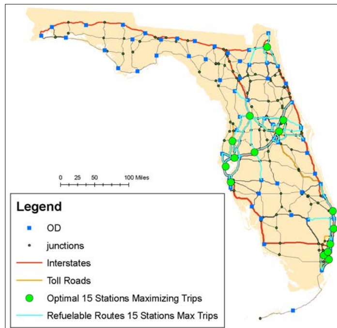
Figure 4.11 Optimal 15 stations maximizing trips with 100-mile working range
