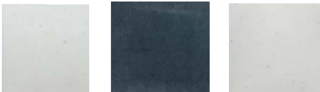
Figure 18. Photos of original (unexposed) (left), exposed to hydrogen (middle) and bleached (6 hrs) (right) samples of AT-Pt pigments.
