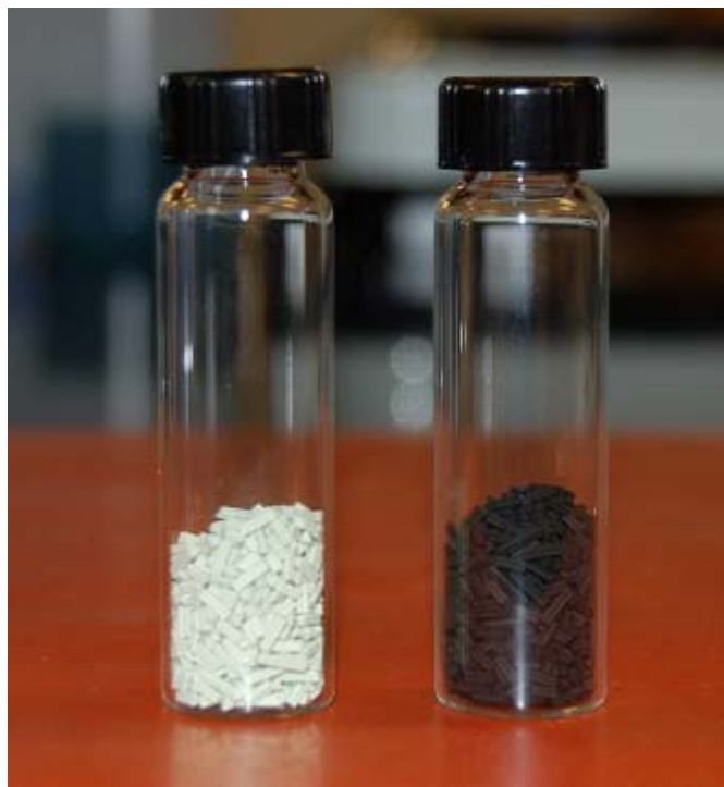
Figure 11. Photograph of Ni-Mo/Alumina catalyst: (left) fresh (in oxide form) (right) after hydro-reforming of high-S diesel (in reduced sulfided form).
