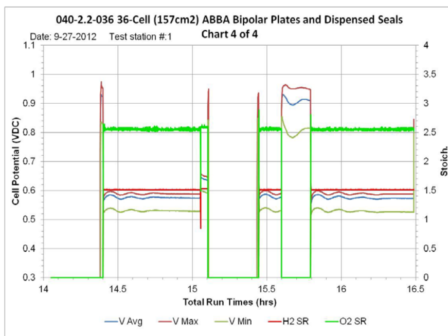
Figure 37. 36-cell stack test data at constant current with 2-phase cooling showing the reactant stoichiometric ratios.
