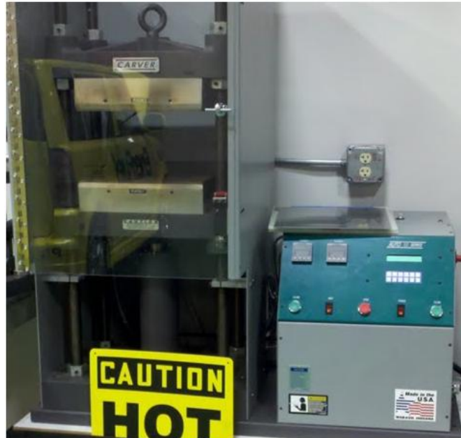
Figure 11. Heated press used to form the HiFoil™ laminates.
