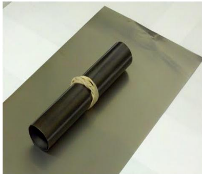
Figure 12. EnerFuel's proprietary high temperature conductive coating comprising graphite and polymer applied to the modified metal foil, and rolled up to demonstrate excellent flexibility.
