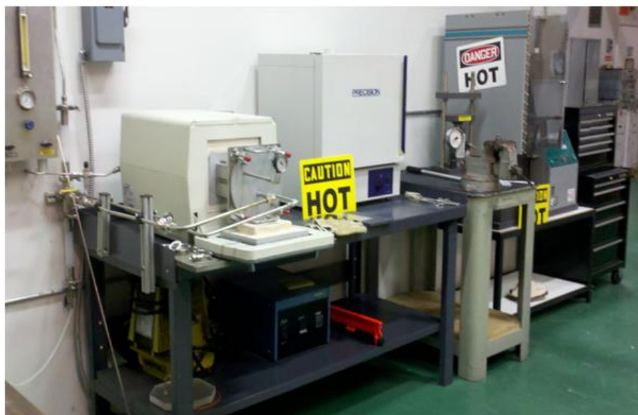
Figure 10. Controlled atmosphere furnace used to bake the conductive coating after application to the metal foil.
