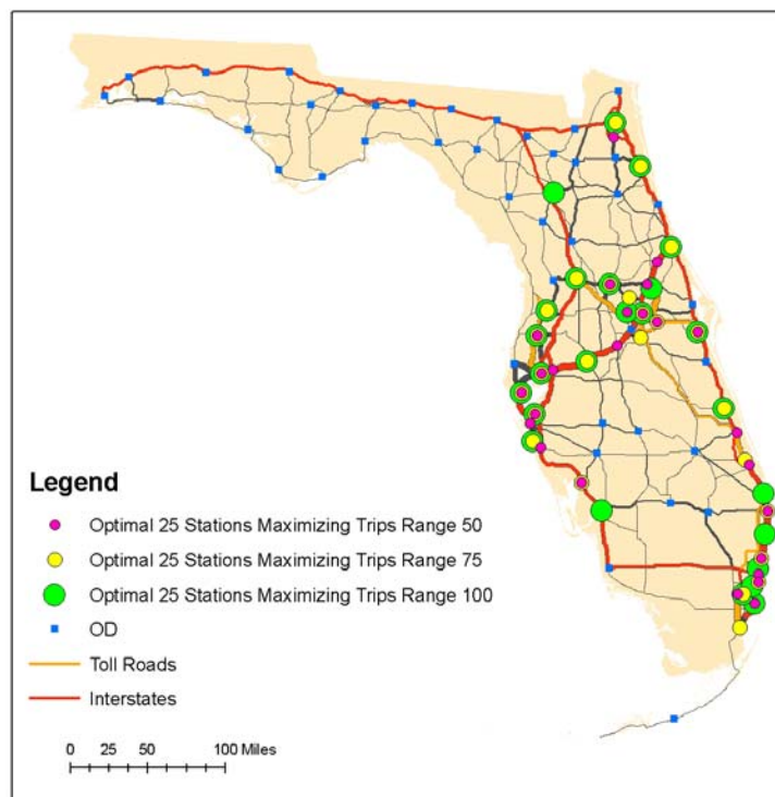
Figure 4.15 Comparison of optimal networks of 25 stations for different vehicle ranges
