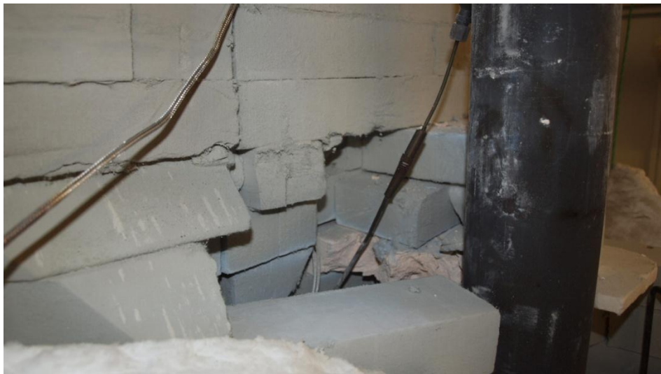
Figure 6-15: Anode inlet thermocouple wire placement.
