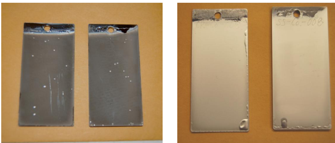
Figure 3-26. Photo on left is as-plated Co on CR-22 (left in both pictures) and SS-441 (right in both pictures) (B). The same coupons after diffusion treatment at 1000° C/4 hours under high vacuum are shown in the photo on right.
