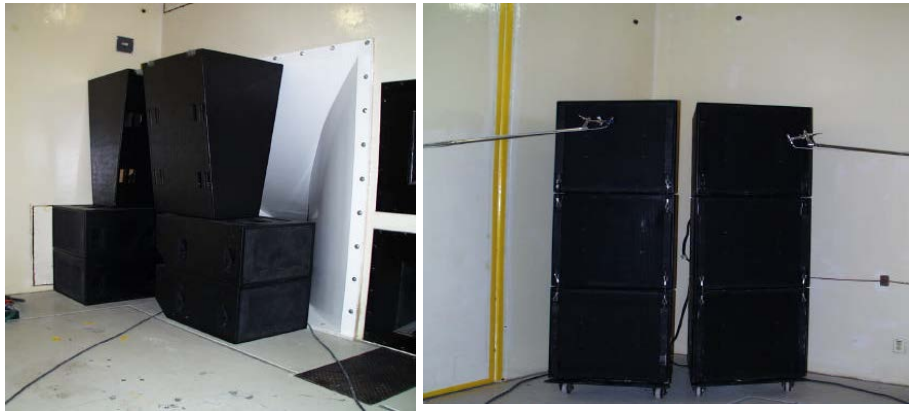
Reverberant Acoustic Field Test (Reverb Chamber)
