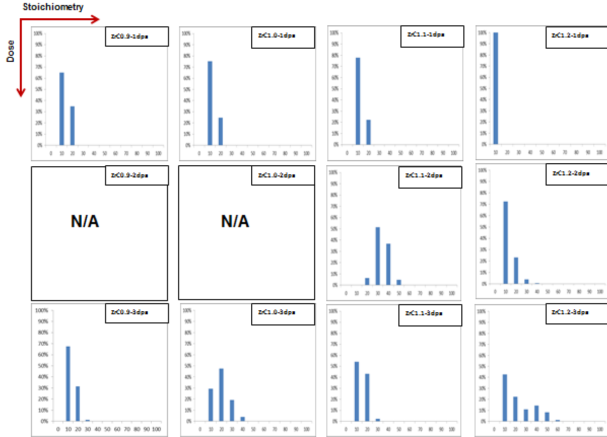
Figure 3.6: Loop size distribution in irradiated \text{ZrC}_x at 400 °C with doses of 1, 2 and 3 dpa.
