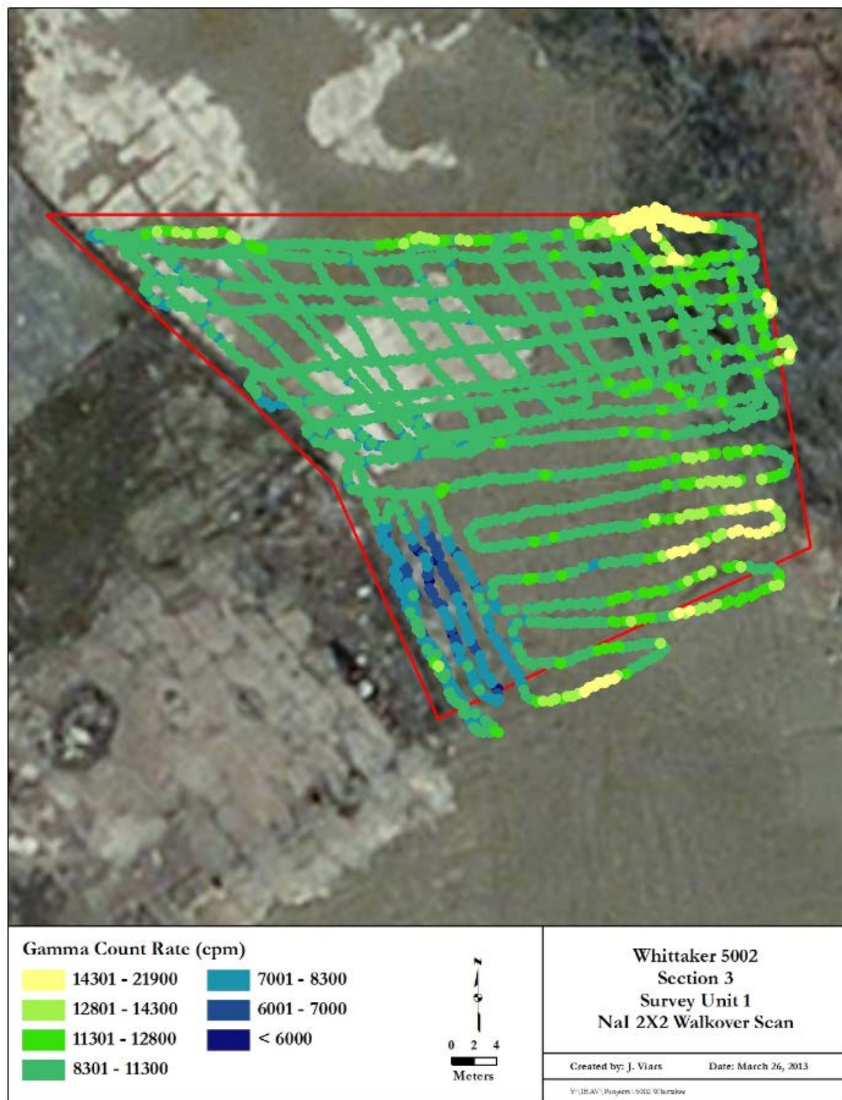
Fig. 3. NaI Gamma Walkover Scan in Whittaker Section 3, Survey Unit 1—Base of Excavation Surface
