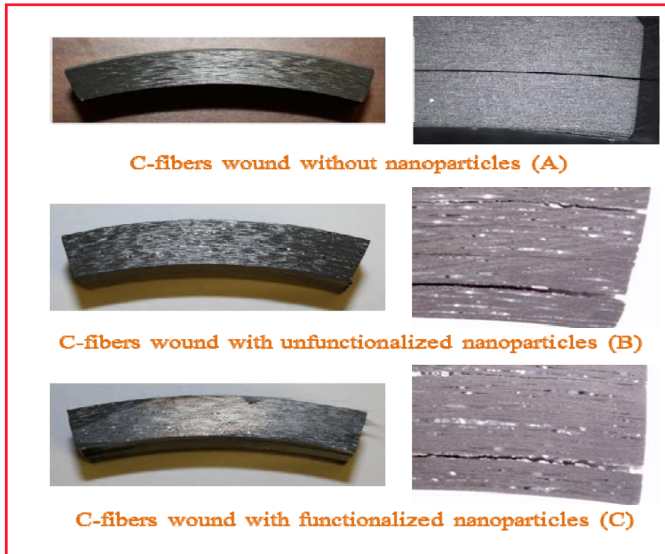
Figure 16. (LEFT) Carbon fiber composite arch samples without (A) and with (B,C) nanoparticles. (RIGHT) Arch composite sample shows interlaminar shear fracture in the center of the sample after testing by 3-point-bend.
