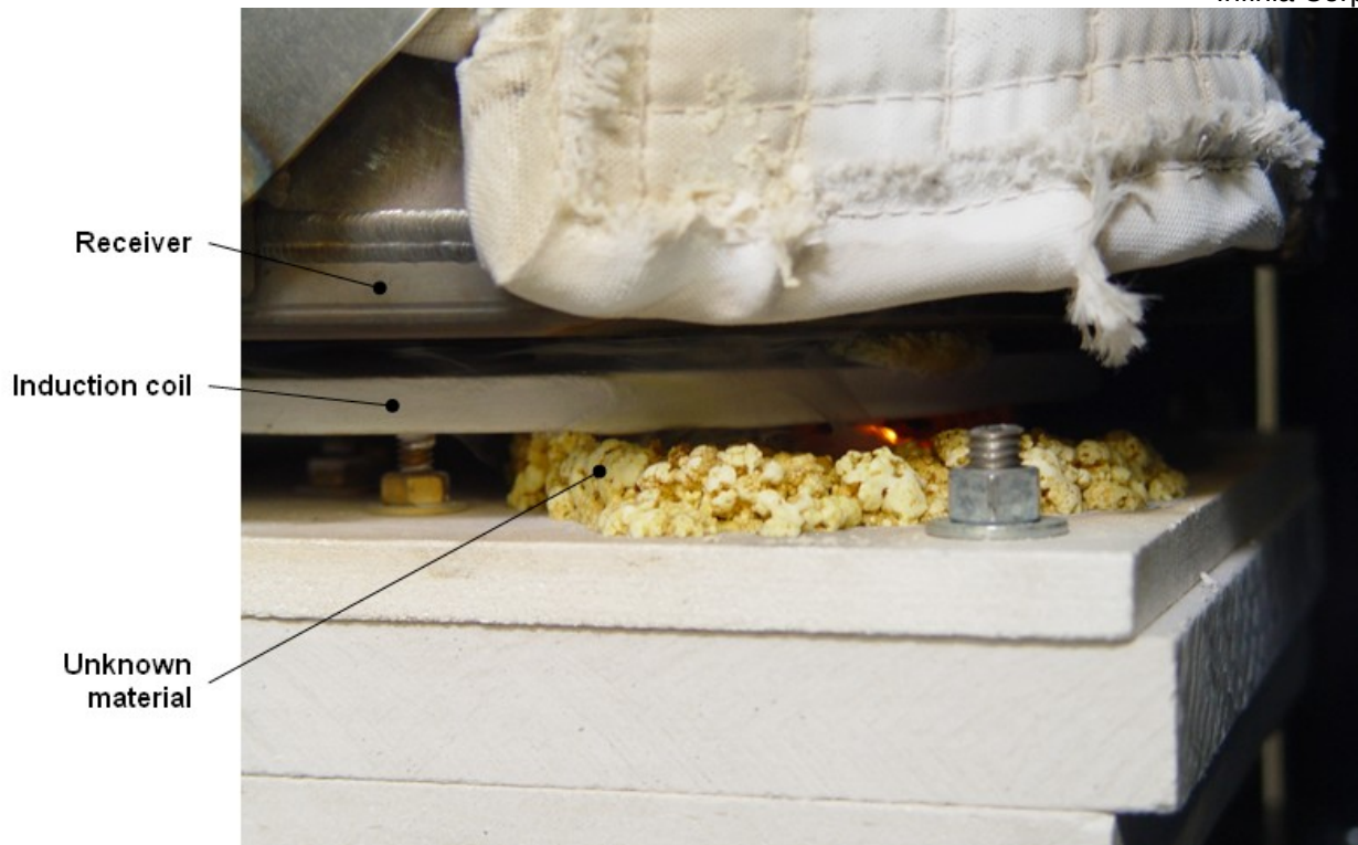
Figure 14, Unknown Material, Post-Failure
