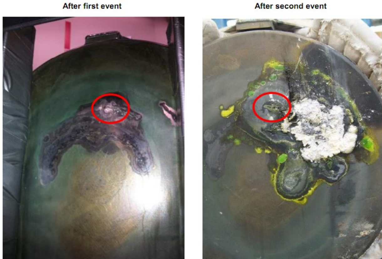
Figure 17, Previous Damage at the Breach Site
