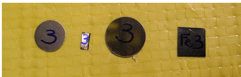
Figure 10. Typical Dosimetry Foils - Left to Right: Co, Sc, Ni, and Fe.
