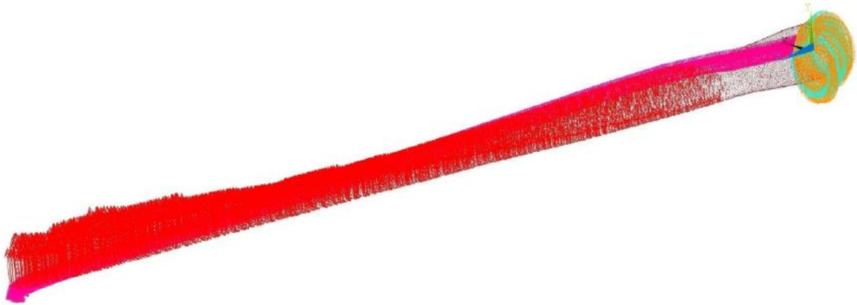
Figure 53. Force vectors representing aerodynamic load applied to the 5-MW blade finite element model
