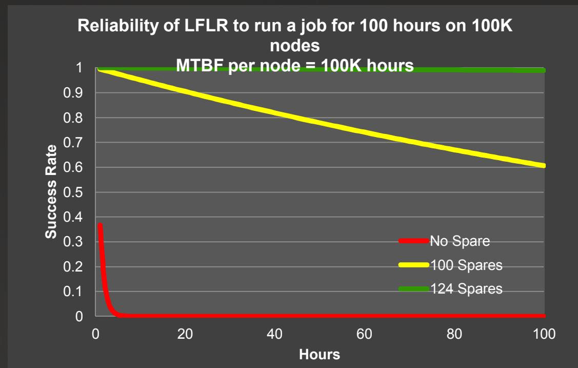
The analytical model shows the probability of a job successfully executing for 100 hours on 100K nodes when the per-node mean time between failure is 100K hours. While the job is nearly guaranteed to have failed after only a few hours when no spares are used, the probability of success is extremely high with only 124 spares.
