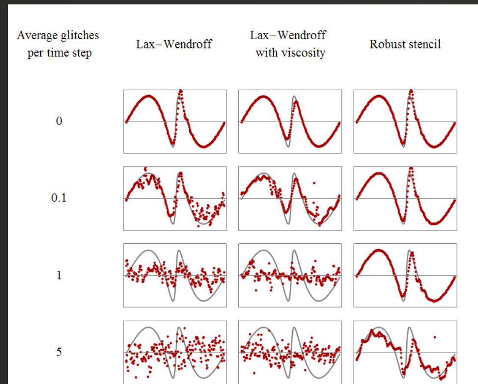
Numerical solution (red points) versus exact solution (gray curve) for a linear advection equation, with various floating-point glitch rates. Small-scale tests more realistic than this demo show the robust stencil tolerates  $\sim 1000\times$  higher silent-error rates than the standard Lax-Wendroff stencil.
