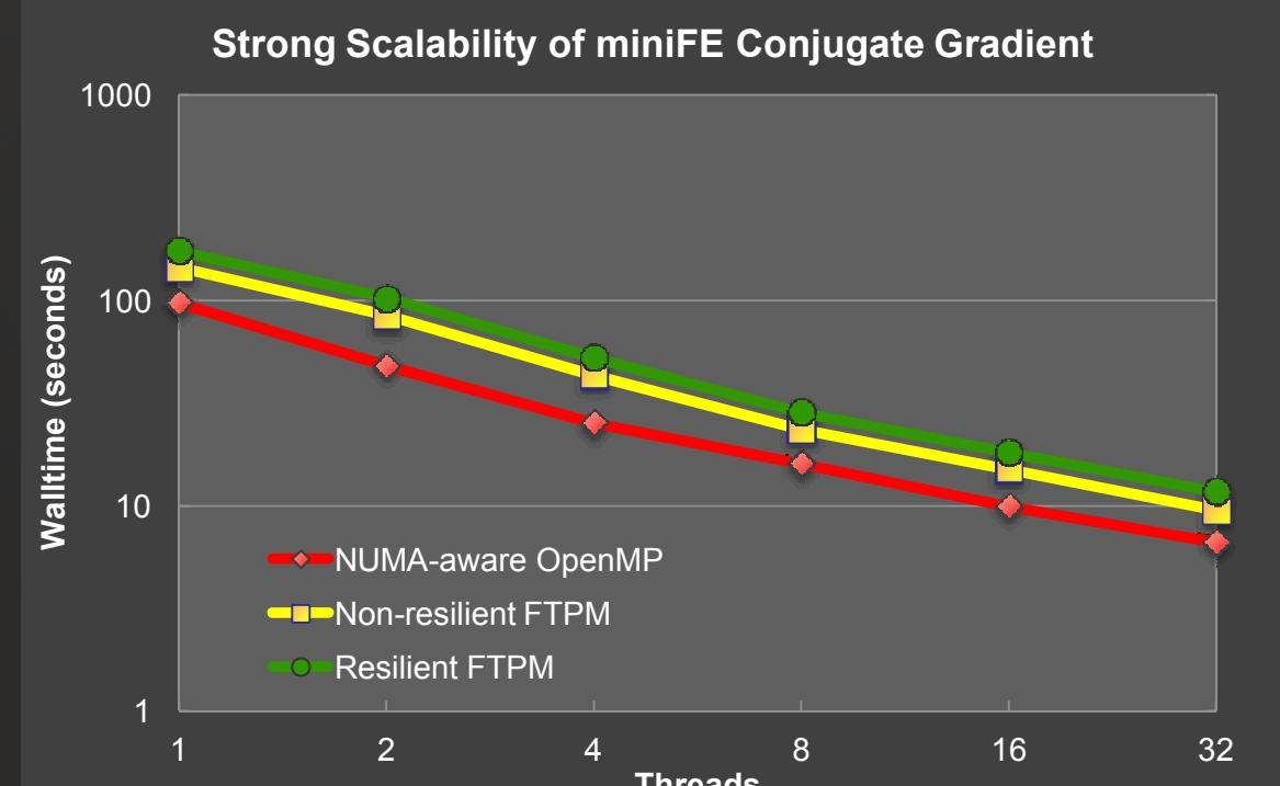
Strong scalability of Sandia's on-node FTPM conjugate gradient port, driven by miniFE, as compared to the Mantevo NUMA-aware OpenMP reference version on a matrix of size 2M with 57M non-zeros. The FTPM code exhibits excellent scalability and competitive performance both without resilience features and with selective resilience.
