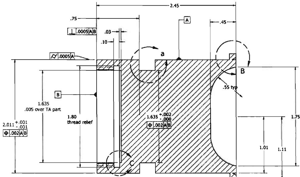
Low impedance material and retaining ring are machined to final thickness
