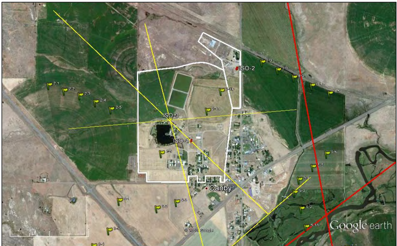
Figure 1 Recommended Drilling ISO-3, flags are MT stations, yellow lines interpreted fault traces.
