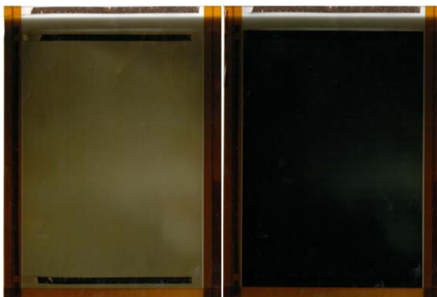
Figure 8: 1,000 cm 2 EC device with Gen 2 materials; critical layers were produced continuously in the 0.5 m tool. Visible light transmission: Dark state of 7% and Light state of 26%.
