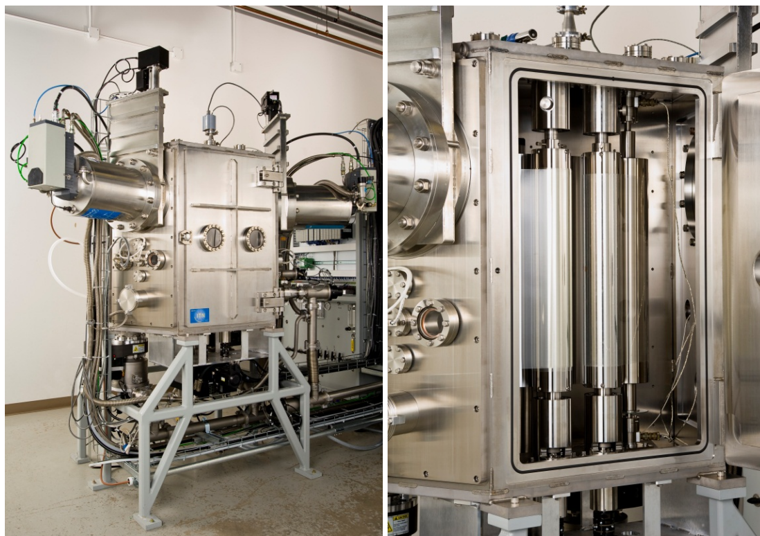
Figure 5. Photographs of ITN's 0.5 meter Pilot Production Tool. There are 4 Deposition Zones, 1 for Each Layer (Transparent Conductor, Electrolyte, Ion Storage, and Electrochromic Layer).
