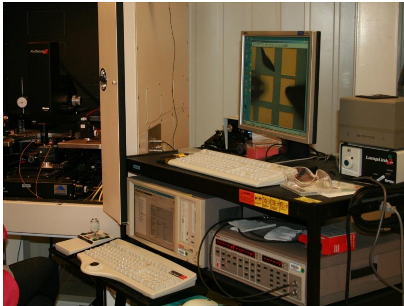
Figure 2: Keithley Semiconductor Characterization Station used to determine electrical properties of TlBr
