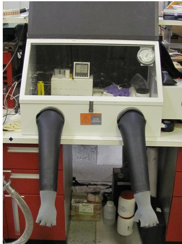
Figure 4: Oxygen Depleted Glove box used to determine the effects of oxygen and humidity on the performance of TIBr detectors
