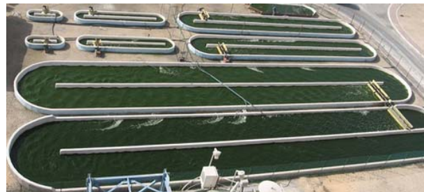
Fig. 1 Conventional algal raceway pond (Photo credit: Seambiotic, Ltd. [5] )
