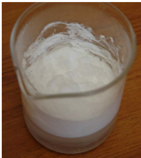
Figure 7. Foam was prepared by aerating 0.5 g of hydrophobic silica nanoparticle (R972, 16 nm) and 50 g of ultrapure water at 14100 rpm in a blender for 180 s.
