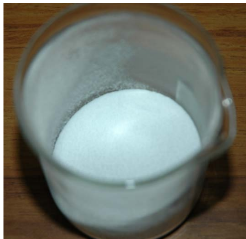
Figure 2. Free-flowing dry water powder prepared by aerating 10.59 g Teflon particle (1 \mu\text{m} ) and 60 g ultrapure water at 14100 rpm in a blender for 180 s.
