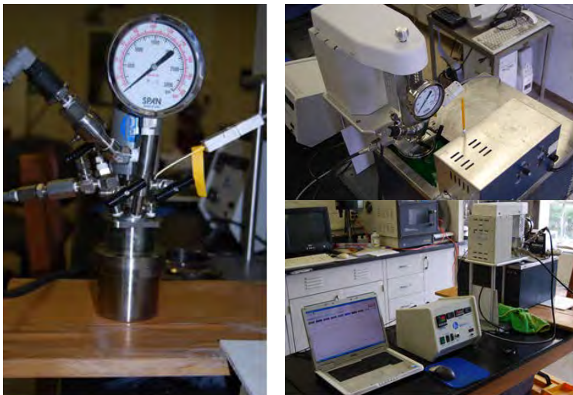
Figure 1. Experimental setup for studying kinetics of gas hydrate formations. Left: 100 ml mini bench top reactor equipped with a RTD probe and a pressure transducer. Right (upper): The temperature is controlled by putting the mini reactor into a refrigerated coolant bath. Right (lower): The temperature and pressure inside the reactor are monitored by a reactor controller and recorded by a computer.
