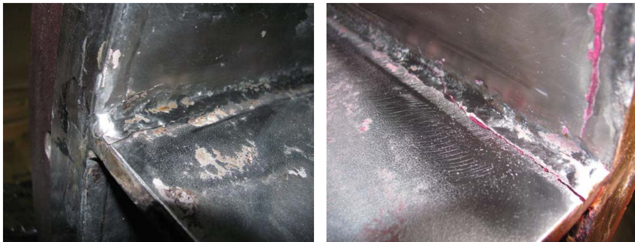
Figure 2. Cracking at the shell / pass partition plate welds.
