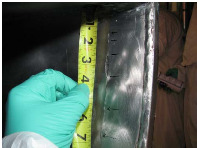
Figure 3. Circumferential, linear indication – affected base metal.
