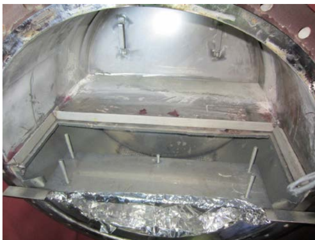
Figure 5. Section of pass partition plate removed – leaving a 3/4-in piece along the shell.
