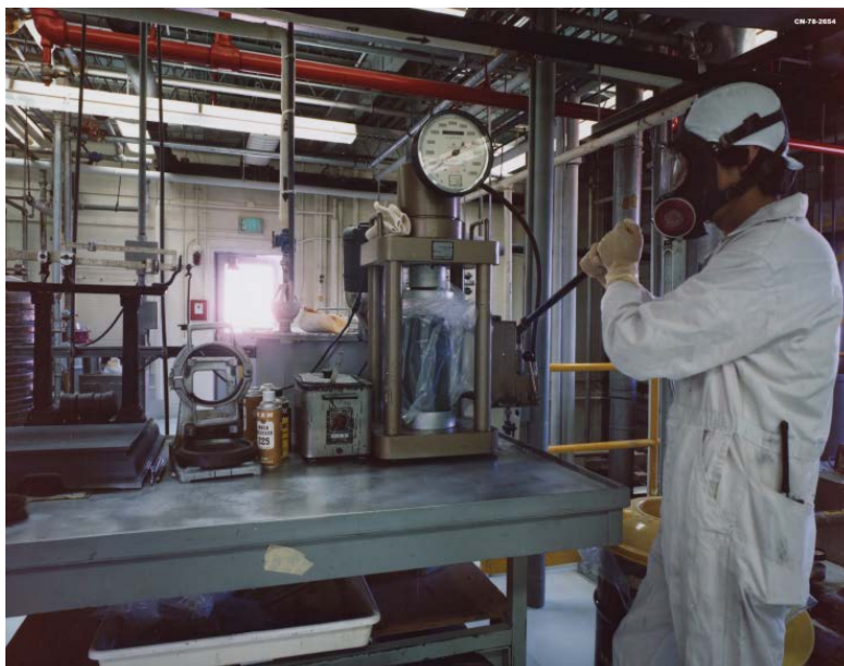
Figure 6. Performing Compression Test on Cured Cement Paste Sample
