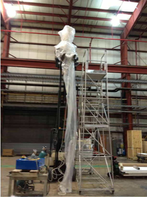
FIG. 36: The ARA completely wrapped to avoid any dust contamination, lifted on the forklift and moving inside a specially assembled long plastic sock that allowed 3-4 meters or telescoping motion.
