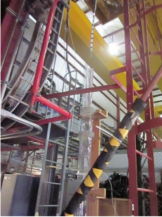
FIG. 27: ARA hanging from the high bay platform above the chimney mock-up.
