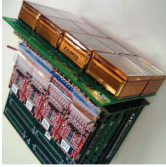
FIG. 6: Compact readout module for the iTOP electronics. This module includes the custom “oscilloscope on a chip” ASIC designed by Varner. The pixelated MCP-PMT photosensors are on the right.
