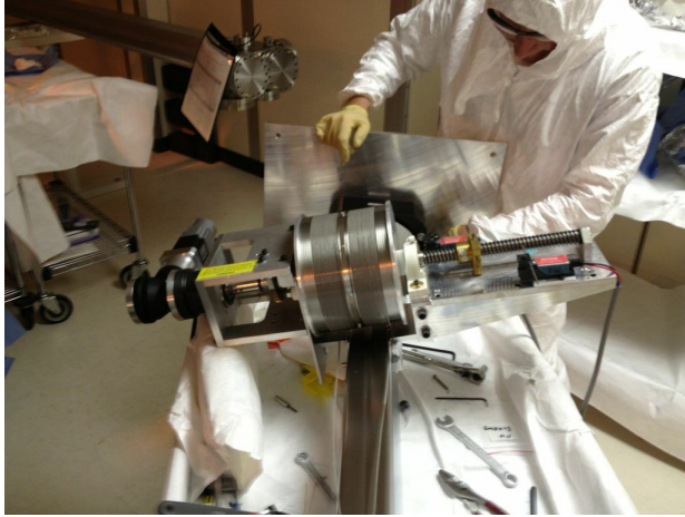
FIG. 34: Clean assembly of the ARA inside the ISO 6 clean room. The ANL technician Frank Skrzecz helping with assembly.
