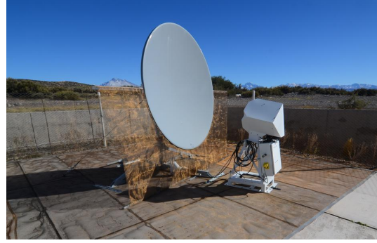
FIG. 54: AMBER installation at Coihueco, Argentina as of March 2013; the bronze mesh screen for reducing thermal noise is evident.
