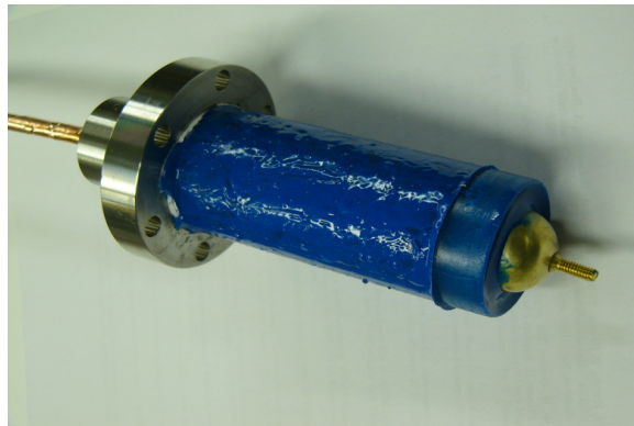
Fig. 5: Photograph of the cathode high voltage feedthrough to be used in our next commissioning run.
