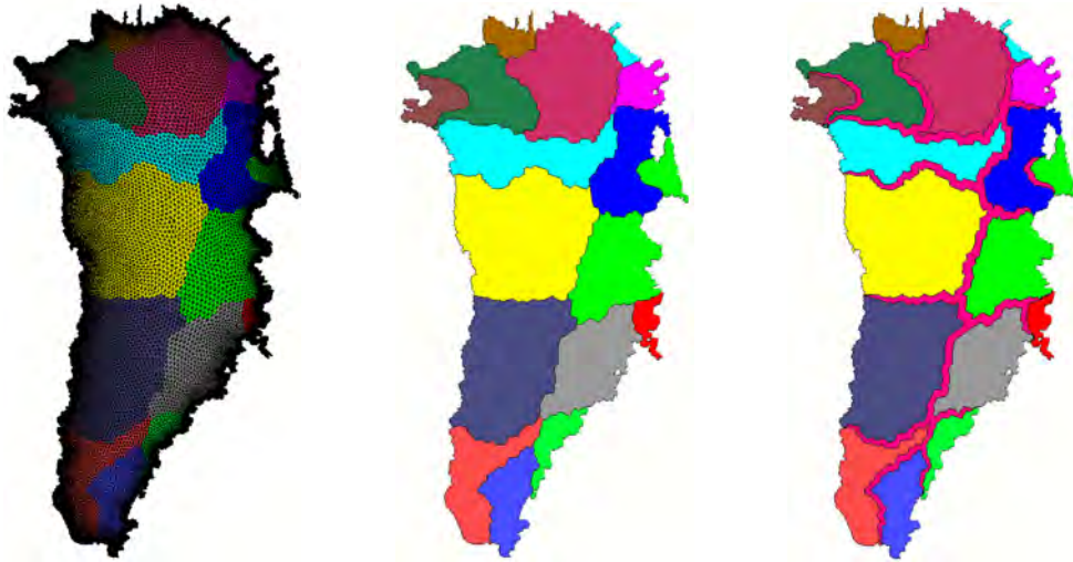
Figure 3: Partition of the Greenland CVDT mesh into 16 sub-meshes and inner boundary formation. Left: the two-dimensional CVDT grid of Greenland. Middle: the mesh is transformed into an unstructured graph which is used as input into the METIS package for partitioning. Right: all sub-domains are expanded by one layer to form the inner interfaces between sub-domains.
