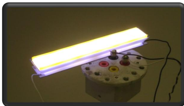
Figure 29. Photographs of linear light engine with >85% total efficiency.
