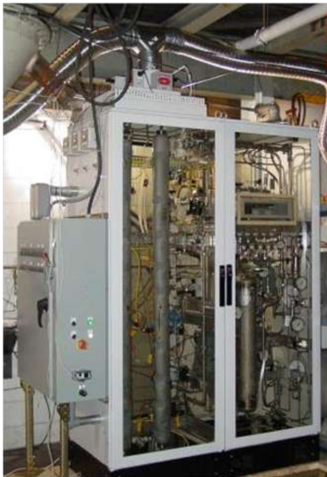
Figure T2-2. Photo of the Sour PSA/TSA Unit.
