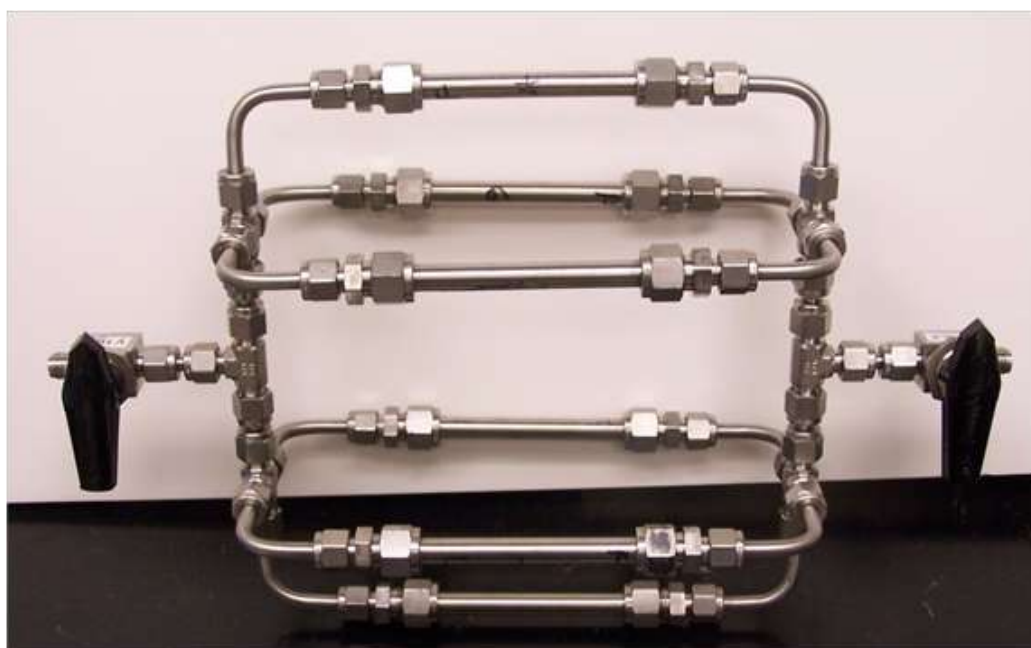
Figure T2-3. Photo of the Six-bed Sour Syngas Exposure Assembly
