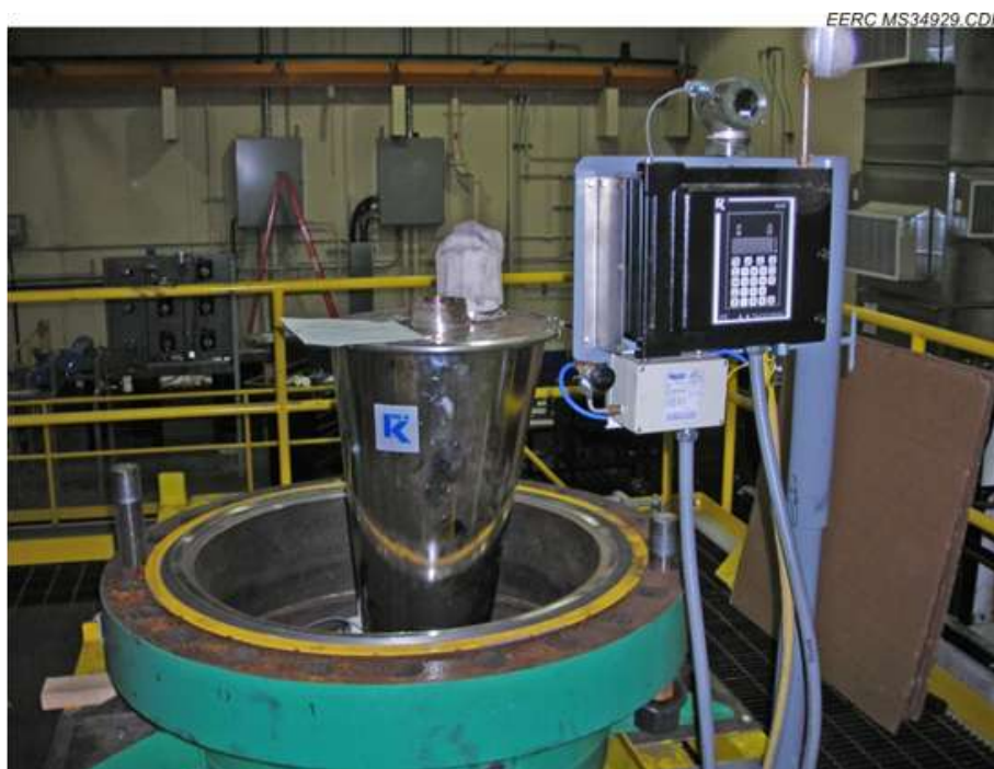
Figure T2-7. Photograph of the fluid-bed coal feed system.
