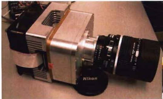
Jan 2005, prototype –in Alu housing Sizable volume taken up by TEC cooler and fan
