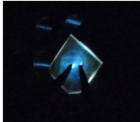
Fig. 70. Demonstration of first blue-wavelength LED on (20-21) GaN substrate.
